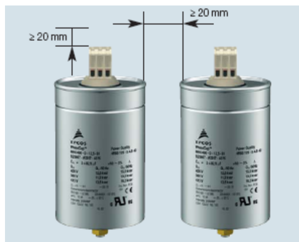
Figure 4: Minimum space over and between the capacitors.
